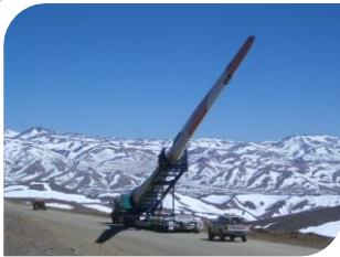
Logistics design, including a hydraulic transportation rig to negotiate the 160km dirt mine track
